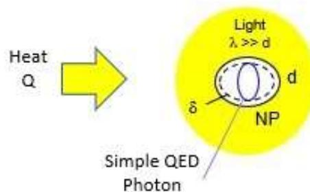
Fig. 5. Heat Q (or light) absorbed in full NP surface
