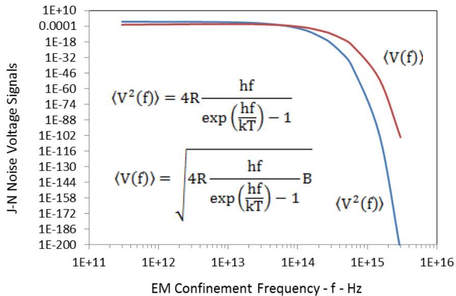
Figure 3 J-N Noise and EM Confinement Frequency
