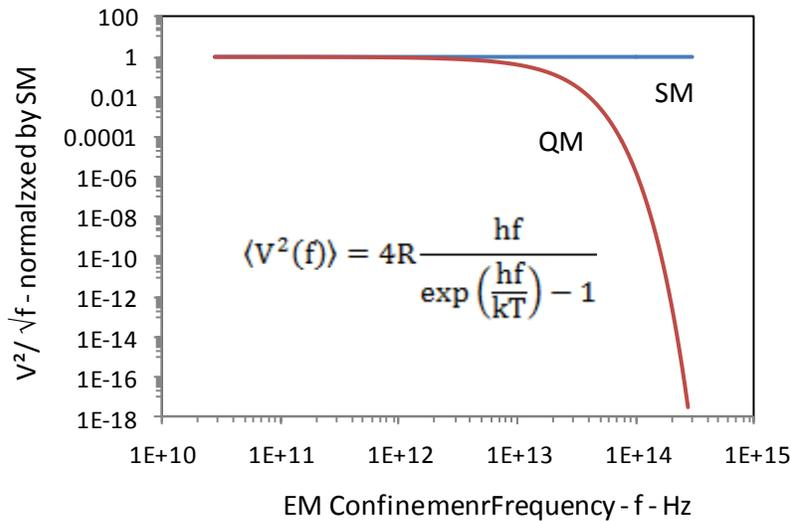
Figure 1 J-N Noise and EM Confinement Frequency
