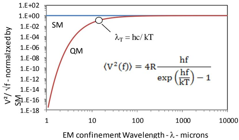
Figure 2 J-N Noise and EM Confinement Wavelength
