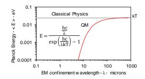
Figure. 2: Planck law of the Atom at 300 °K In the inset, E is Planck energy, h Planck's constant, c light speed, k Boltzmann's constant, T temperature, and  $\lambda$  the EM confinement wavelength
