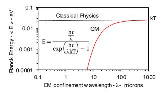
Fig. 4: Planck law of the Atom at 300 °K In the inset, E is Planck energy, h Planck's constant, c light speed, k Boltzmann's constant, T temperature, and  $\lambda$  the EM confinement wavelength
