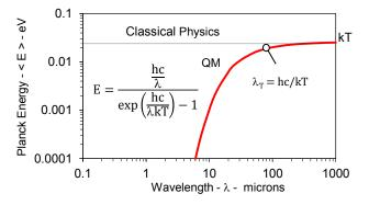
Figure 1 Planck energy of the atom at 300 K
