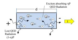
Fig. 2 Memristor - Charge Distribution - Positive Voltage Bias
