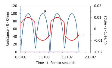
Fig. 3 Transient Resistance R and Current I at 1 GHz
