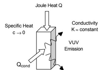
Zero specific heat means the thermal diffusivity diverges. Conductivity measurements by the Pulse method based on diffusivity are therefore unstable, the stability achieved by inclusion of the substrate in diffusivity measurements.
