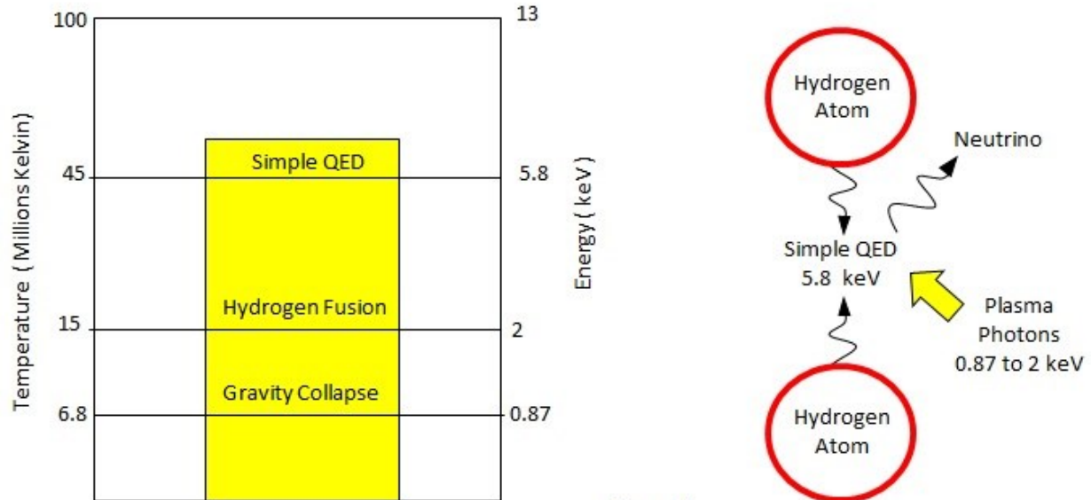
Figure 2 Simple QED Fusion and approach of Hydrogen Atoms
