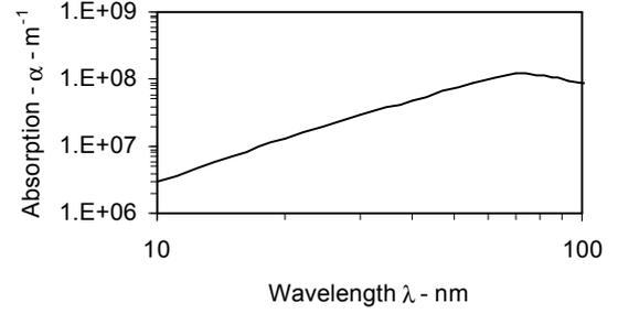
Fig. 4 – Absorption of Water at 300K.
