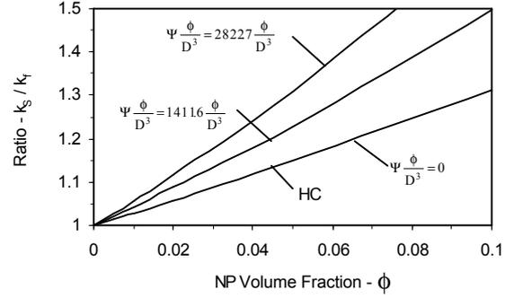
Fig. 6 – QED Effect on HC Thermal Conductivity
