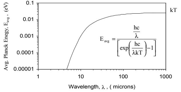
Fig. 2 – Planck Energy of Harmonic Oscillator at 300K. In the inset,  $k$  is Boltzmann's constant, and  $T$  is temperature
