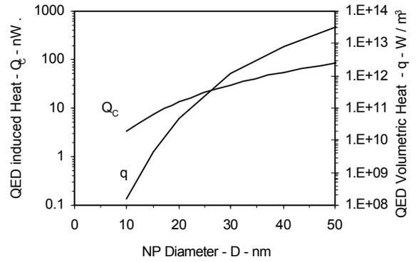
Fig. 5 – Collision Heat  $Q_C$  and Volumetric  $q$  Heating
