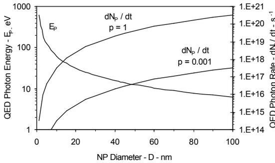
Fig. 3 – QED Photons and Rate induced in NP
