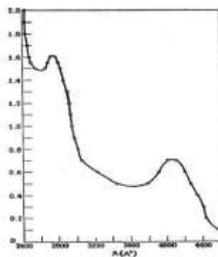
Figure 8. Catalase UV absorption spectra
