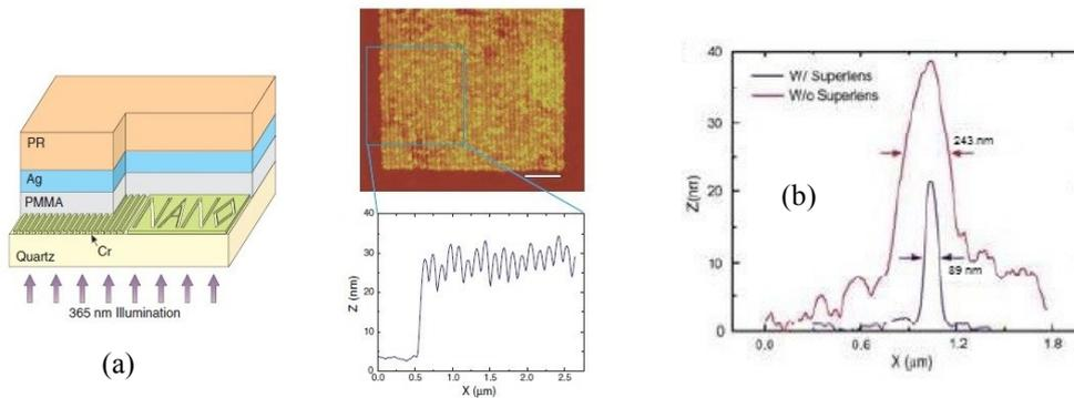
Fig. 2. Superlens Configuration and Enhanced Image Quality
