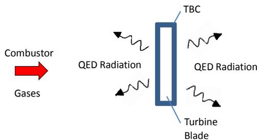
Fig. 1 QED Cooling Turbine Blade and submicron TBCs
