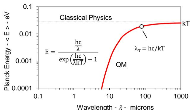
Fig. 1 Heat Capacity of the Atom at 300K
